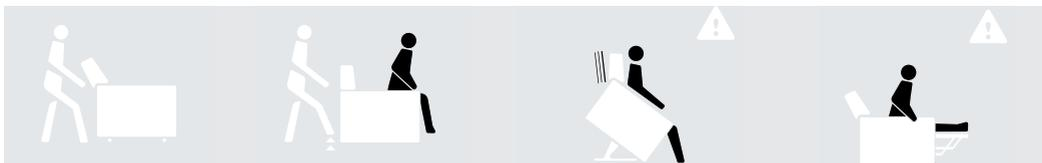
Unlock the roller system only when the armchair is unoccupied.
